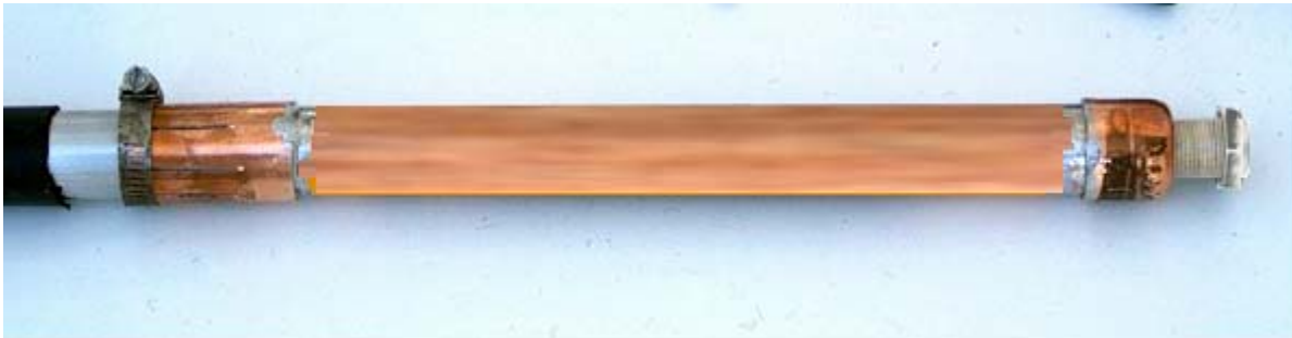
Figure 3. The completed transformer. (the N connector nut is not screwed in)
