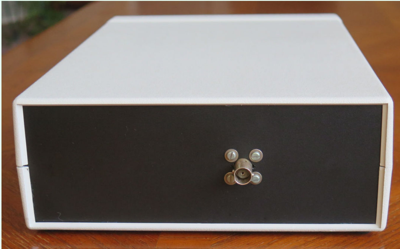
The balun is built in a plastic case (Hammond 1598JSGYPBK)
