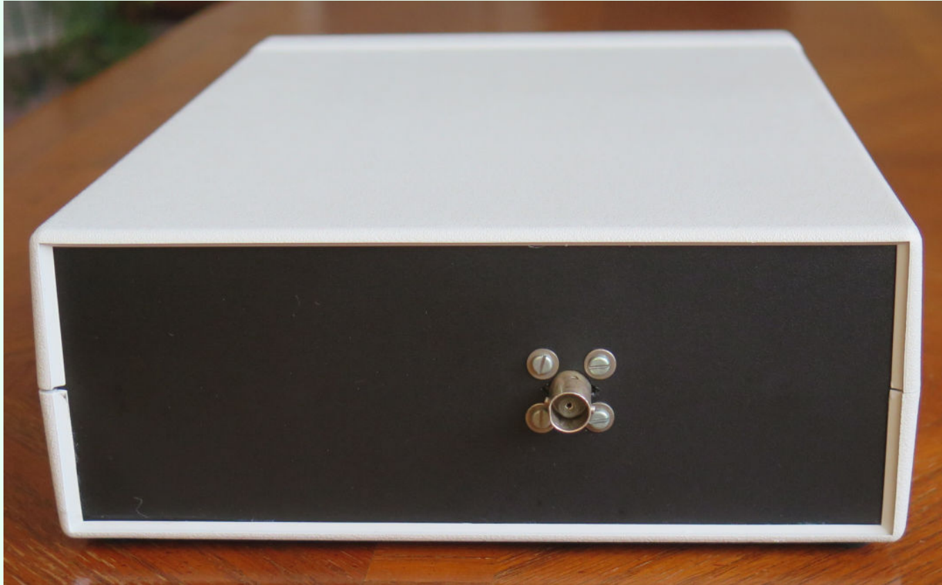
The balun is built in a plastic case (Hammond 1598JSGYPBK)
