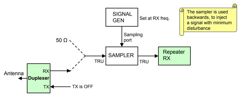
Adjust Sig Gen to check sensitivity with 50  $\Omega$  term connected. Repeat sensitivity test with Antenna connected (Connect to duplexer RX port) With the antenna, the sensitivity is degraded by the antenna noise present. Note the reduction.
