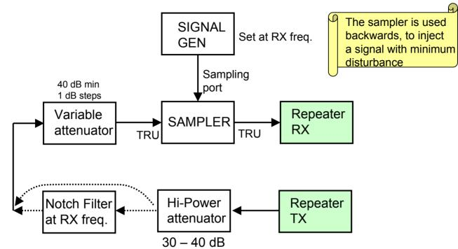
Set up equipment as shown.
