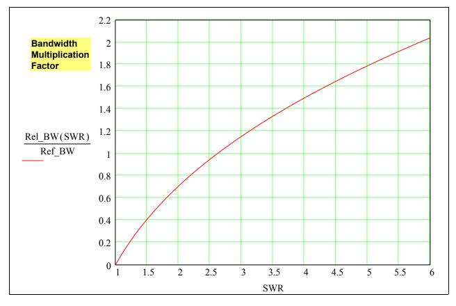
For SWR = 2, the BW is 0.707 times the BW at the reference SWR of 2.618
