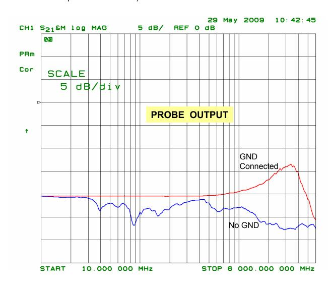
**Probe Output**: The probe signal is monitored while the trace is terminated in 50  $\Omega$
